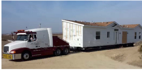
(Left) Completed modular house components in the factory lot and in transit to the project site.
