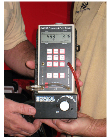
(Above) Meter reading of final Blower Door test showing 376 cu. ft. per minute at the blower door fan with 50 pascals of pressure in the house, converting to 1.12 air changes per hour (1.12 ACH50).
